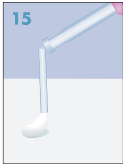
Gently dispense a small amount of core-x™ flow onto a mixing pad DO NOT USE EXCESSIVE FORCE!
