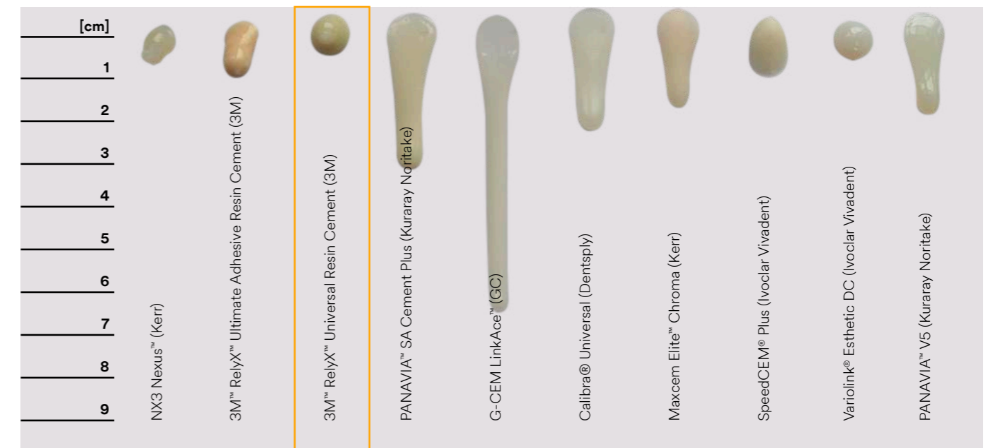
Fig. 2: To compare the flow properties, equal amounts of each cement were applied on a pad which was stored upright at 36°C/96.8°C for 2 minutes before the cement was light-cured. Source: 3M internal data
