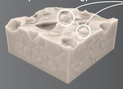
As the resin wears, large and unevenly sized filler particles are exposed. This creates a rough and uneven surface as they break away from the resin matrix.
