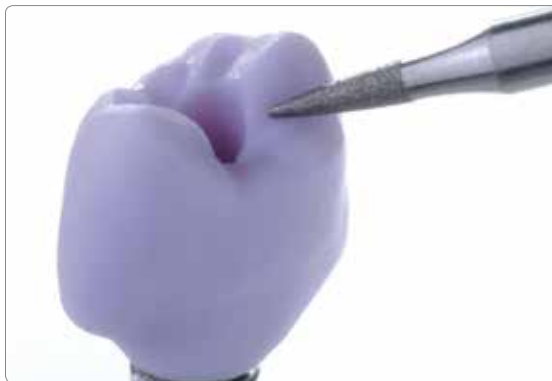
The surface of the ceramic structure is ground with a fine diamond to smooth out the surface structure created by the CAD/CAM procedure.
