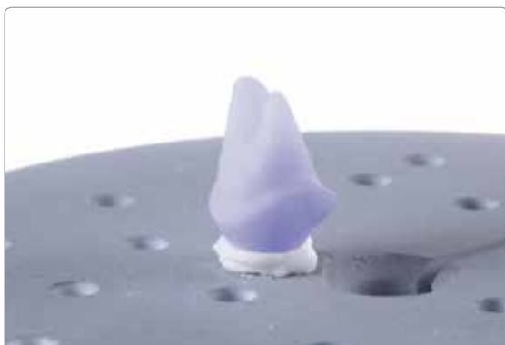
The interface of the ceramic structure is slightly overfilled with IPS Object Fix Putty or Flow. Then the ceramic structure is placed in the centre on the IPS e.max CAD Crystallization Tray.
