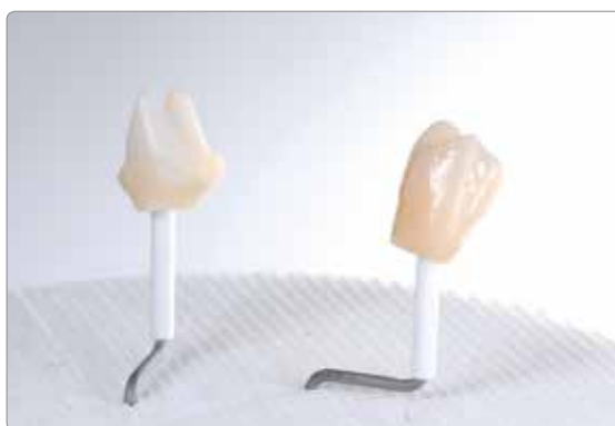
The Stain and Characterization firing is conducted on a honey-comb firing tray.
