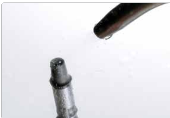
Removal of the silicone and subsequently cleaning with ultrasound in a water bath or with the steam jet.
