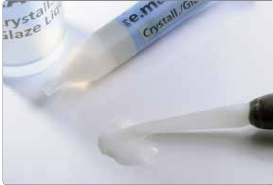
IPS e.max CAD Crystall./Glaze Paste is extruded from the syringe and mixed. If required, the paste can be thinned with IPS e.max CAD Crystall./Glaze Liquid.
