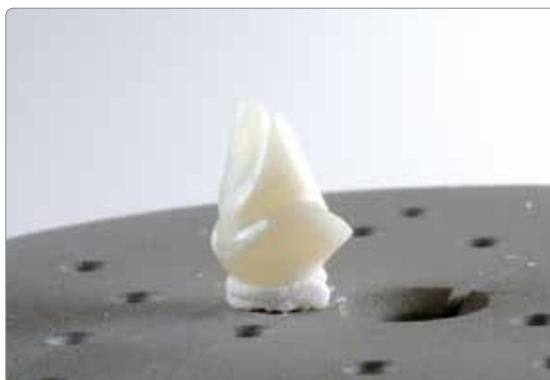
The crystallization tray is removed from the furnace once the crystallization program has been completed and the object is allowed to cool
