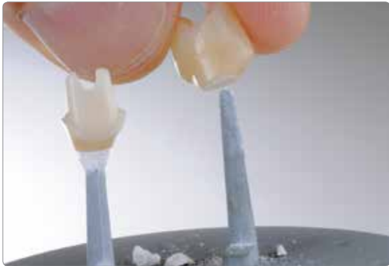
The ceramic structure is removed from the IPS e.max CAD Crystallization Pin XS.
