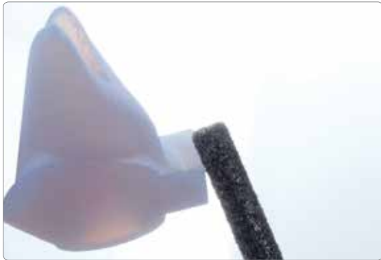
The attachment point to the block is smoothed out taking the shape of the emergence profile and the crown margin into account.
