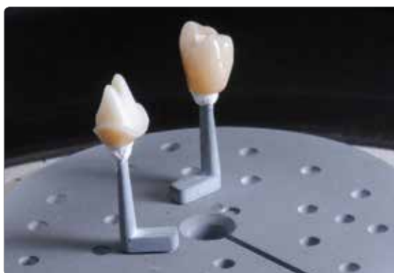
The ceramic structure is removed from the furnace after completion of the firing cycle (wait for the acoustic signal of the furnace).
