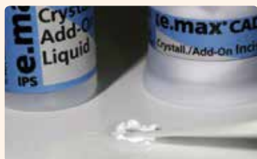
Mixing IPS e.max CAD Crystall./Add-On with IPS e.max CAD Crystall./Add-On Liquid to an easy-to-contour consistency
